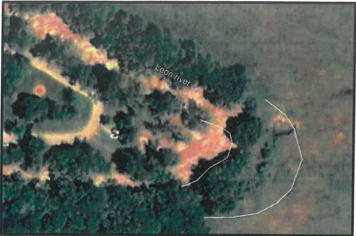
Figure 3: 2004 Aerial photo with Figure 2's tops of left and right embankment superimposed. The river has moved away from the park notably between 2004 and 2022. Similar findings were noted at other meanders (bends in the river) near the park.
